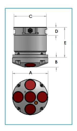
Face view and Side view of 5 beam system. Size of each transducer is 2 inches.
